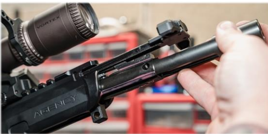
STEP 9: DEPRESS REAR TAKEDOWN PIN, CONNECTING UPPER WITH LOWER
