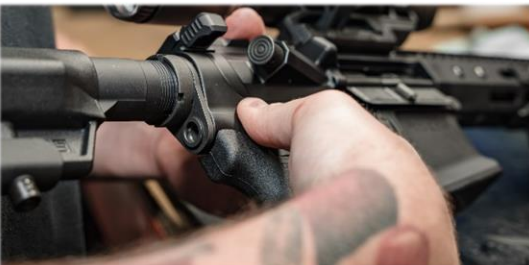
STEP 9: DEPRESS REAR TAKEDOWN PIN, CONNECTING UPPER WITH LOWER
