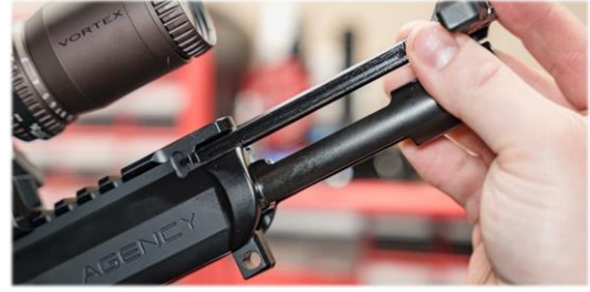
STEP 6: APPLY LUBE TO CONTACT SURFACES OF CHARGING HANDLE
