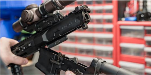
STEP 5: APPLY LUBE TO CONTACT SURFACES OF BCG
